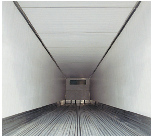
Liner/Scuff panels are impact & abrasion resistant, easily cleaned and resist attack from a wide range of chemicals.
