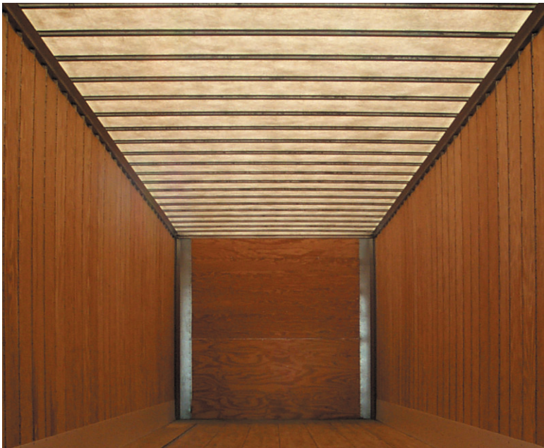
UV stabilized translucent roofs let natural light into the trailer allowing for safe and easy loading and unloading of freight.
